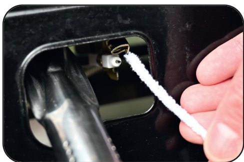
Cleaning of the pilot flame conductor with a chenille wire or a pipe cleaner.
