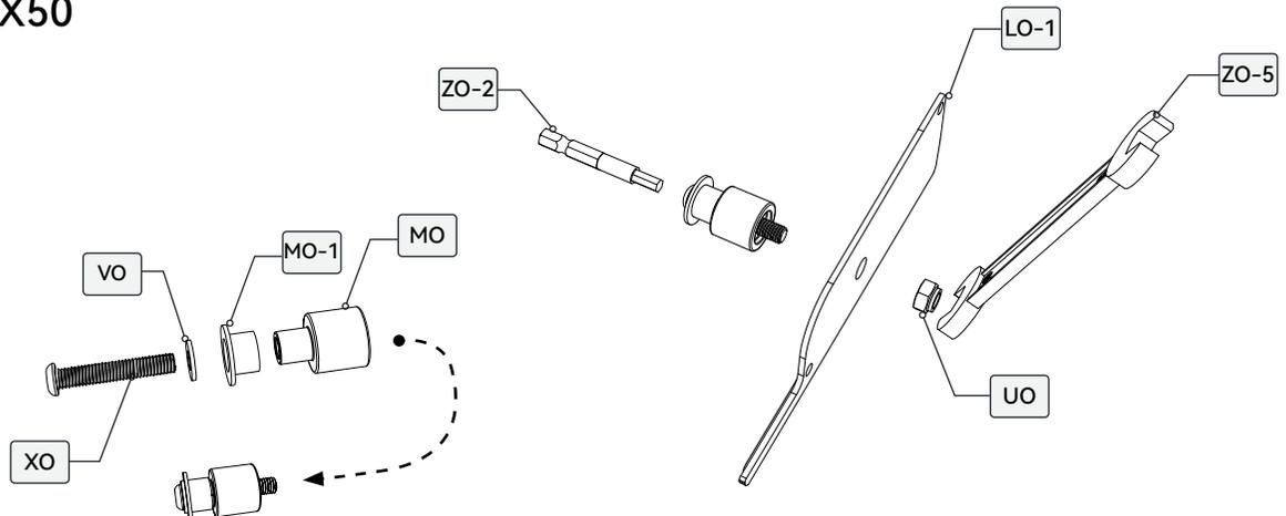
Install the louvre cover on two ends of the installed louvres and the spindle louver.
