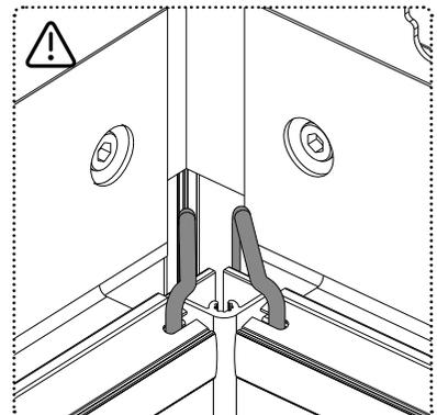
Install the main shaft louvers and secure them using screws. Ensure that the louvers are level.
