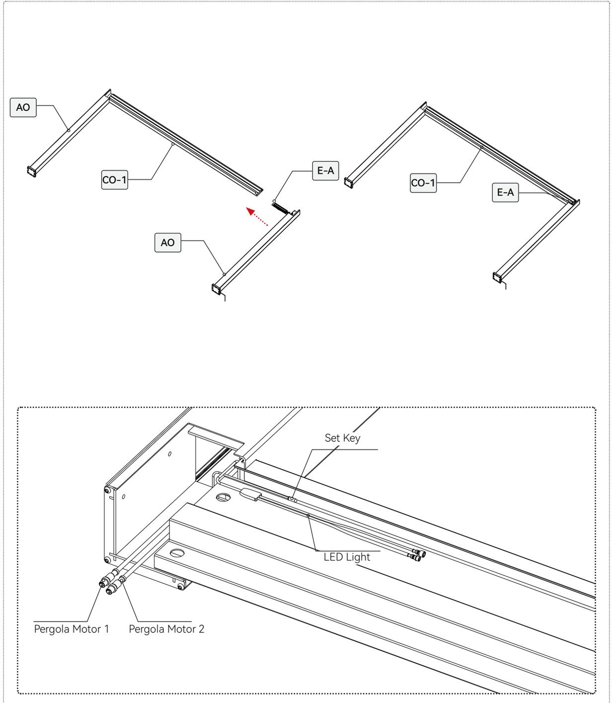
Install the screws for the side beams.
