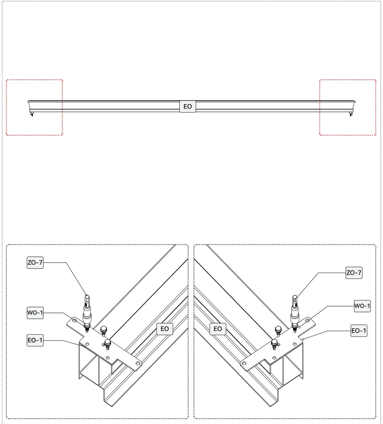
Secure the intermediate beam to the intermediate column using provided fasteners, ensuring proper alignment, stability, and correct placement of the beam.
