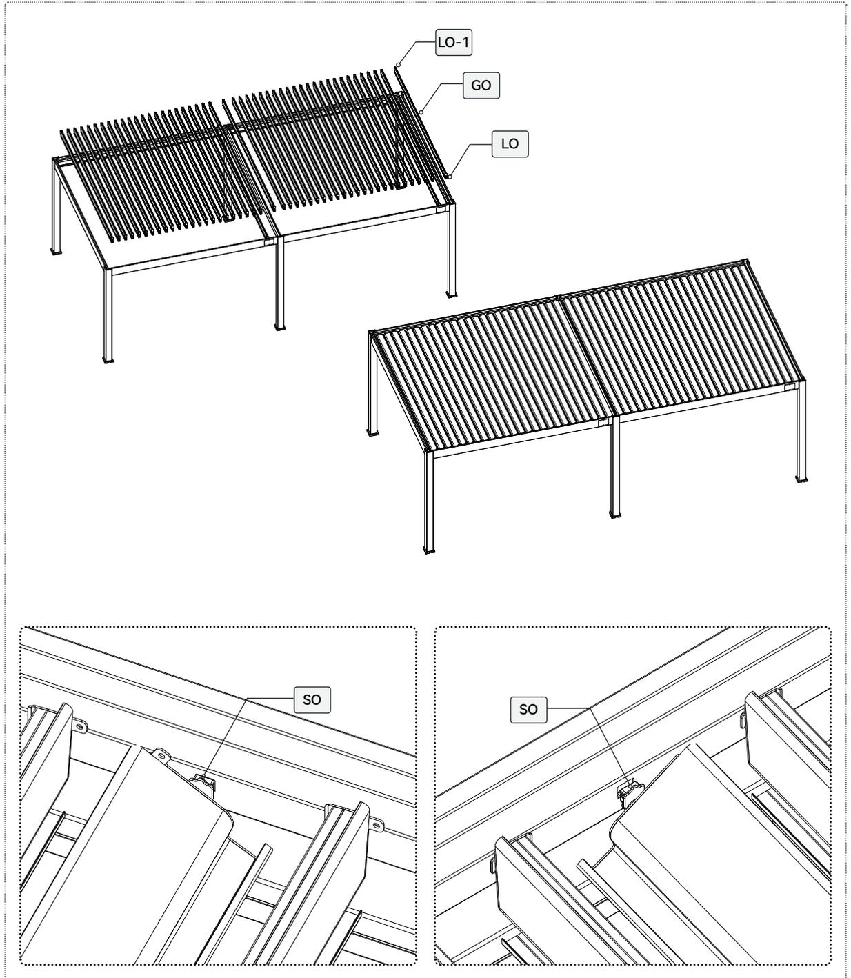
Complete the connection of the connecting rod:
